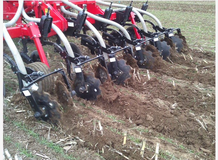
Strip-till/sweep injection (DSI with paired disks – “Clozr”)
