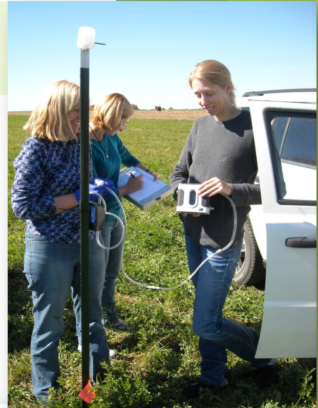
Field air flow calibration
