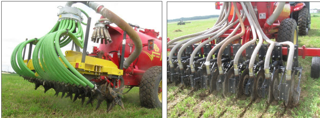
Figure 1. Aerator/banded manure (Aerway SSD; left) and shallow injection (Yetter Avenger; right) application implements.
