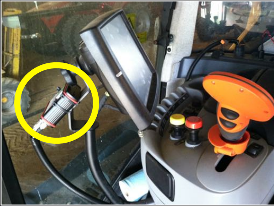
CANcaseXL installed behind monitor in harvester.
