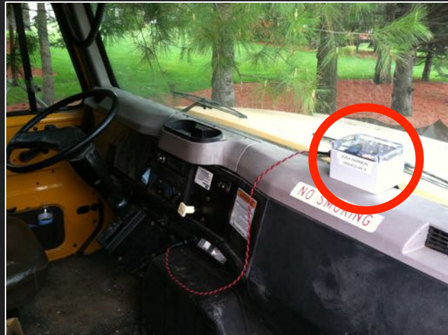
Arduino loggers installed in cabs of trucks.
