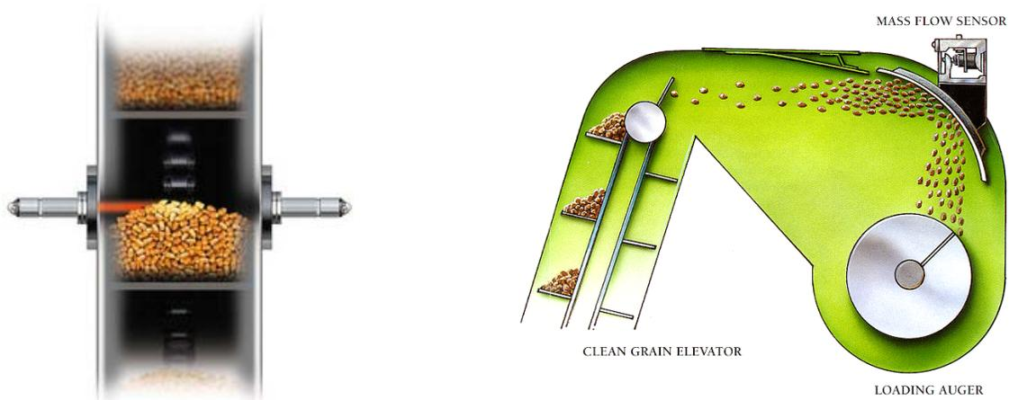
Figure 1: Volumetric (left) and impact plate (right) mass flow sensors <sup>3</sup>.
