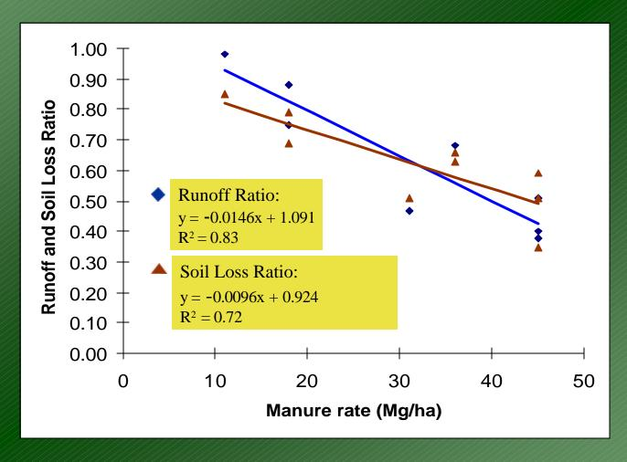
adapted from Gilley and Risse (2000); slope length 20-40 m; gradient 4-13%
