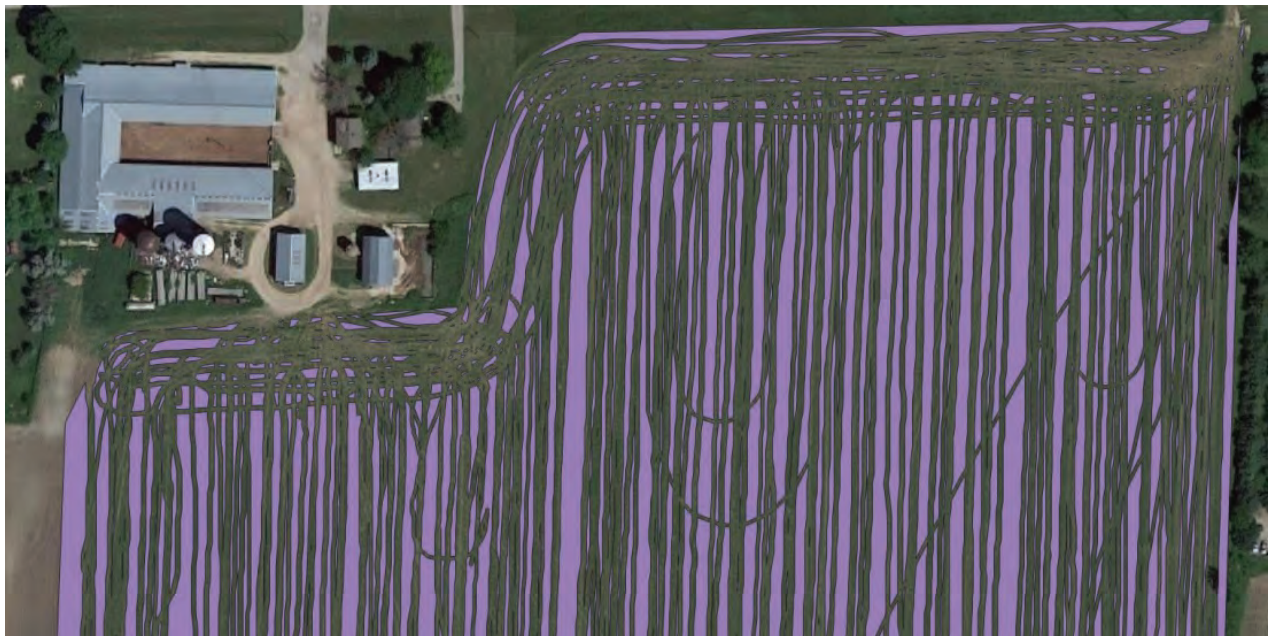
Figure 2. Area of field covered (green) by wheel traffic based on machinery footprints.
